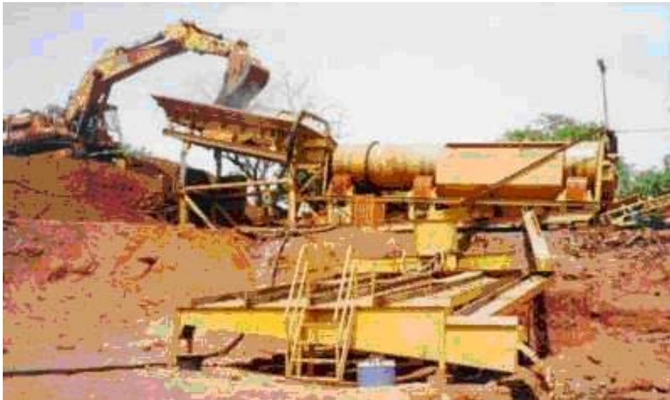
Figure 2.2. Photo of a typical wash processing plant for gold consisting of a grizzly, trommel, and sluice recovery system (e-goldprospecting.com).
